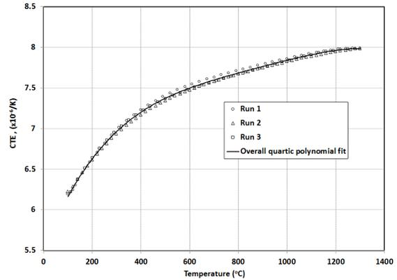
Figure 3 Measured CTE for three runs on the DIL806
