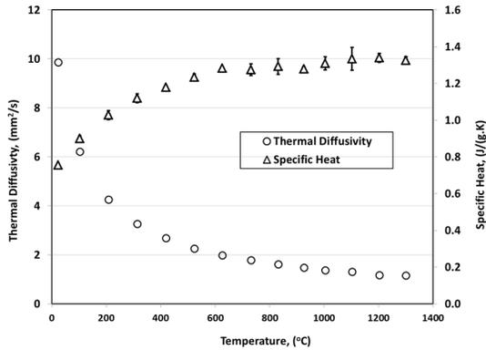
Figure 4 Thermal diffusivity and specific heat results of the unknown alumina sample, the error bars are the standard deviations of the values by three laser shots.
