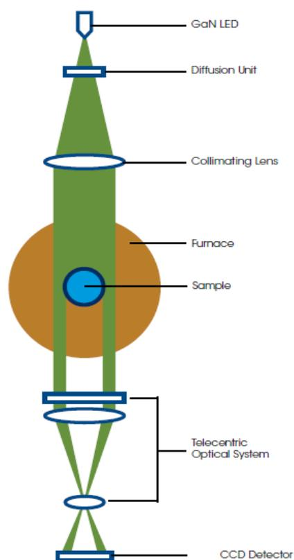
Figure 1 Schematic of the DIL806
