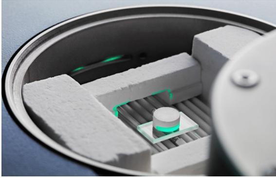
Figure 2 The furnace of the DIL806 in open status
