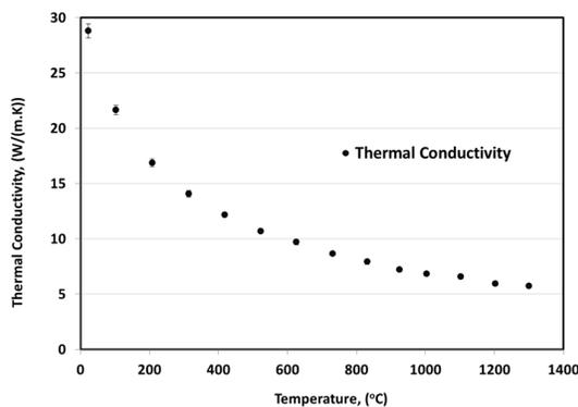
Figure 5 Calculated thermal conductivity of the unknown alumina sample, the error bars are the standard deviations of the values by three laser shots.
